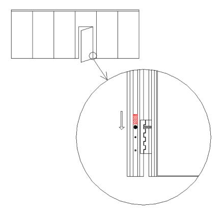
• Set up the rest of the wall. The last panel is the telescopic panel and has a part that extends to seal the wall sideways.
