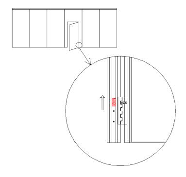
• Release the panels at the edge of the frame, important to turn until the push beams are fully retracted.
